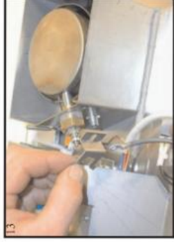
13 Remove the glow plug retaining plate and negative grounding wire.
