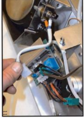
11 Disconnect the glow plug connection cable.
