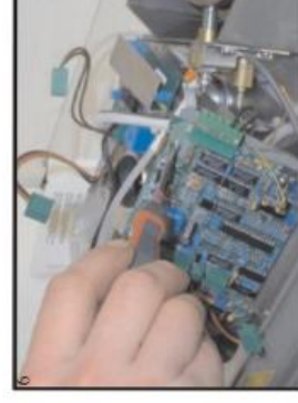
Remove the circuit board retaining screw.
