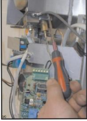
8 Remove the screw holding the T4 thermostat retaining plate.
