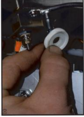
10 Remove the gasket which seals the T4 thermostat.
