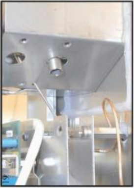
(View of the partially extracted fuel needle.)
