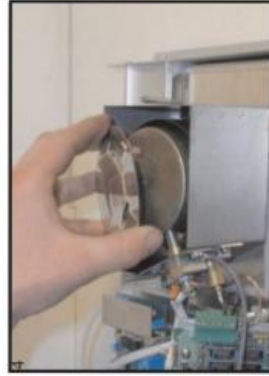
Remove the burner pot retaining spring plate.
