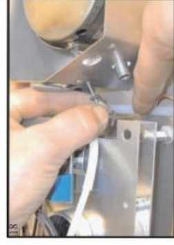
18 Extract the fuel needle far enough to be able to remove the burner assembly. (If the fuel needle is partially or fully blocked with carbon then remove and replace.)
