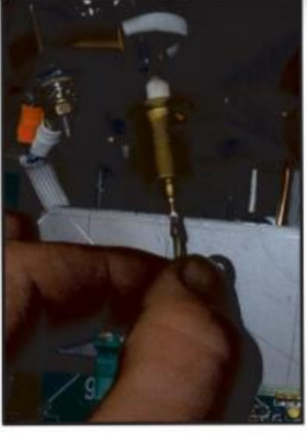
9 Remove the T4 thermostat and retaining plate.
