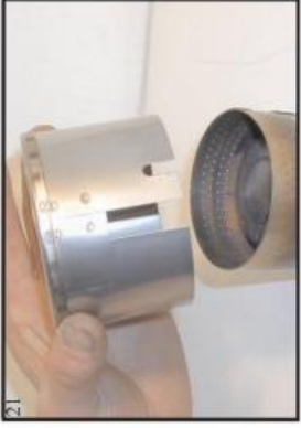
Lift and remove heat shield from burner.
