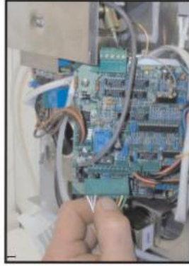
Remove the control panel connection plug. (grip all coloured cables firmly so as not to pull on single cables.)
