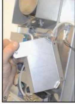
16 Remove PCB retaining plate
