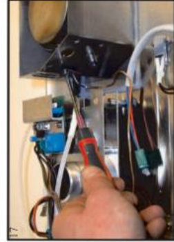
17 Remove the screw which holds the fuel needle retaining plate.
