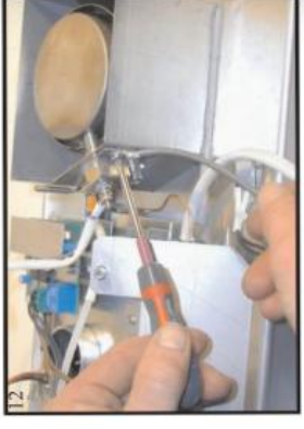
12 Remove the screw which holds the negative grounding cable and glow plug retaining plate.
