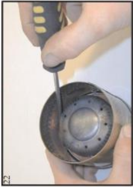
Using a flat blade screw driver compress the retaining spring to release the flame spreader.
