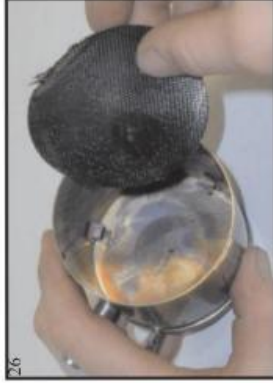
Remove the quartz bottom carpet. Clean the carbon deposits from the burner. If the carbon can be removed from the quartz carpet with out damaging it then reinstall, if not then replace it with new.
