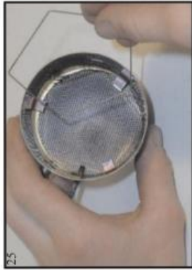
Remove the quartz bottom carpet retaining spring.
