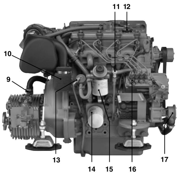
D2-75 with reverse gear MS25L
