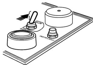
3. Push the rocker switch to the "Glow" position. The indicator light comes on and the glow plugs are connected to pre-heat the engine. Let the glow plugs remain activated for 10 seconds (max. 30 seconds).
