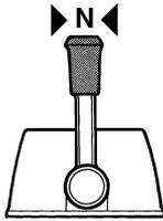
1. **If the engine is cold:** Disconnect the gear shift function and move the control lever forwards to half throttle.
