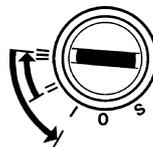
4. Turn the key to position "III" to start. Release the key as soon as the engine has started, the key will automatically spring back to the "I" position. If the engine did not start the key must first be turned to the "0" position before trying again.
