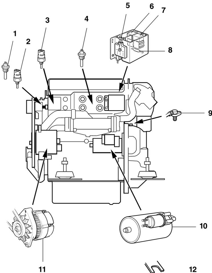
1. Engine coolant temperature sensor D2-55 (optional extra)
