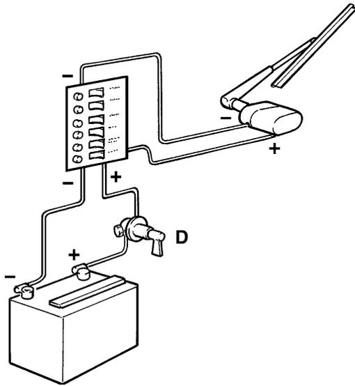
5. If an auxiliary battery is in use, a main switch (D) should be connected between its + terminal and the fuse block. The main switch for the auxiliary battery must cut off all power consuming equipment connected to that battery and be turned off when power is no longer needed.
