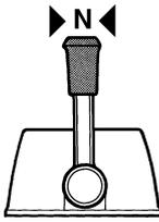
1. **If the engine is cold:** Disconnect the gear shift function and move the control lever forwards to half throttle.
