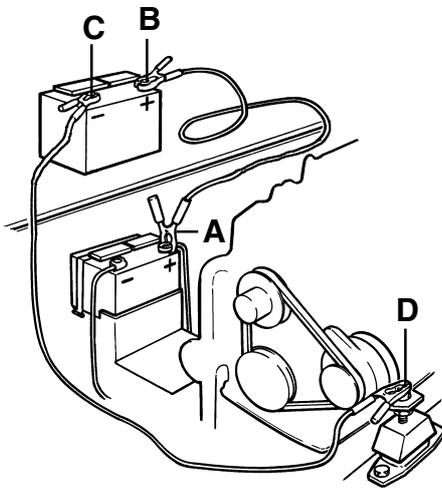
1. Check the auxiliary batteries have the same rated voltage as the engine's system voltage.
