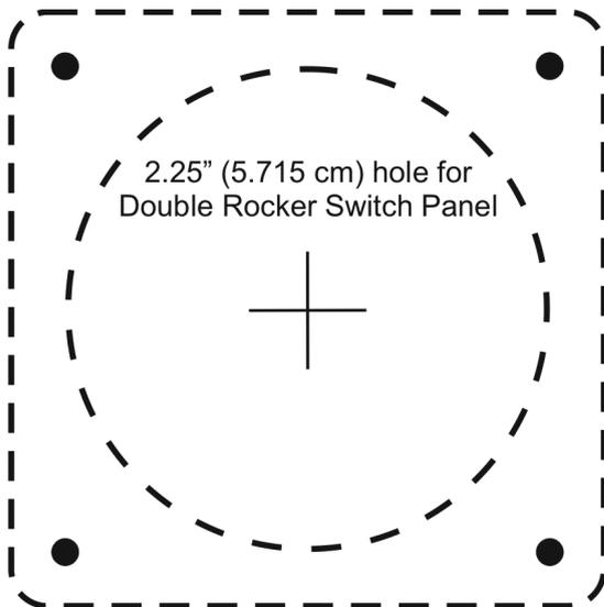
Remove the template from the owner's manual by cutting around the dashed rectangular perimeter line.
