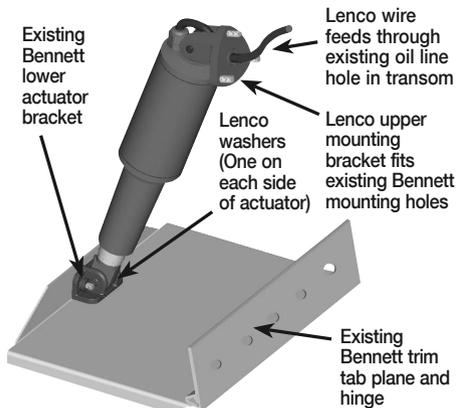
We recommend using 3M 5200 adhesive caulking to bed the upper mounting bracket and screws.
