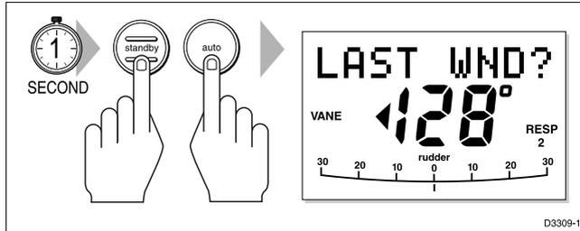
The LAST WND? text alternates with the previous wind angle and direction. The previous locked heading is displayed, with an indicator to show you the direction in which the vessel will turn.
