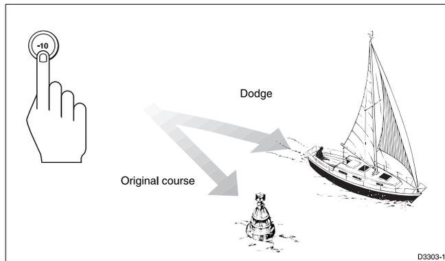
When safely clear of the obstacle, you can reverse the previous course change (for example, press **+10** three times), or return to the previous locked heading (LAST HDG).
