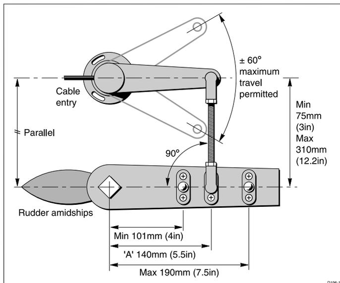
2. Dimension **A** should, ideally, be 140 mm (5.5 in) – changes within the limits shown will not degrade the autopilot performance but will slightly alter the scaling of the rudder angle display.
