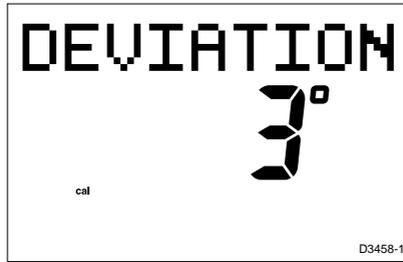
This shows the maximum deviation detected, and indicates that compass correction has been completed successfully.
