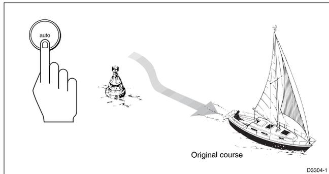
If you do not press **auto** while the display is flashing, the current heading will be maintained.
