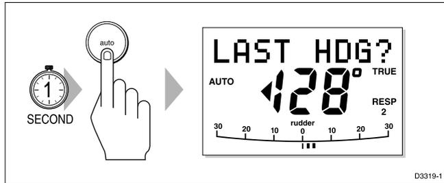
**Note:** A direction-to-steer indicator is displayed to show you the direction the vessel will turn.
