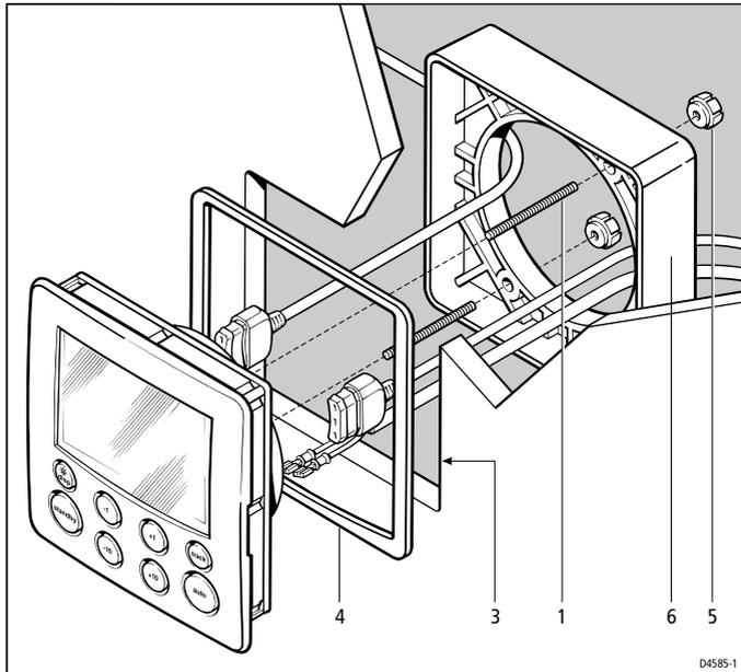
5. Screw the two fixing studs (1) into the threaded sockets on the rear of the control head.
