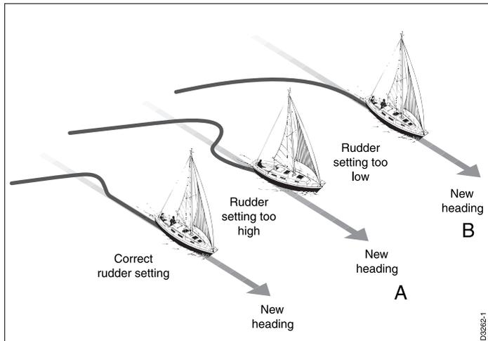
These actions are most easily recognised in calm sea conditions where wave action does not mask basic steering performance.
