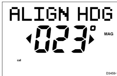
8. Use the **+1** and **+1**, keys, or the **+10** and **-10** keys, to increase or decrease the displayed heading, until it agrees with the ship's steering compass or a known transit bearing.
