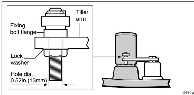
1. Using the adaptor pin supplied, make sure the pushrod ball is attached to the tiller arm with its flange positioned between the ball end and the tiller arm.
