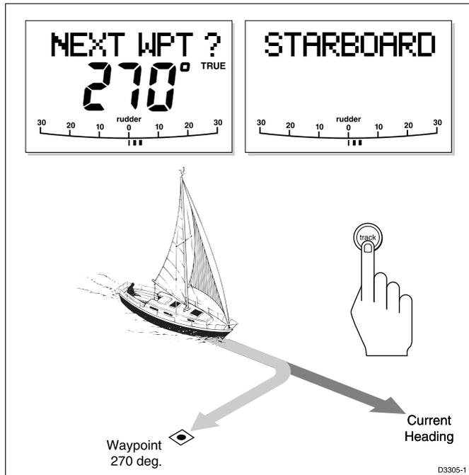
**Note:** *If the vessel is further than 0.3 nm from the track, the Large Cross Track Error alarm will sound. Press **standby** to cancel the alarm, hand steer closer to the track, and press **auto** and **track** again.*
