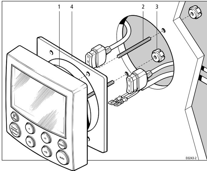
3. Drill two 4 mm (5/32 in) diameter holes for the fixing studs.
