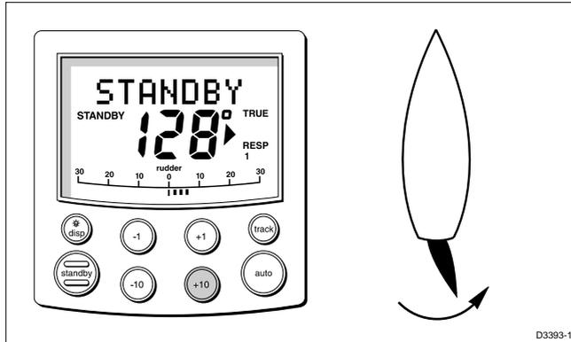
3. If the helm produces a turn to port, reverse the drive connections on the back of the control head.
